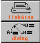
PRINTER. Printing the whole file (e. g .part program) or only marked file parts from the EDITOR. It is possible if the printer is connected to the system only.
