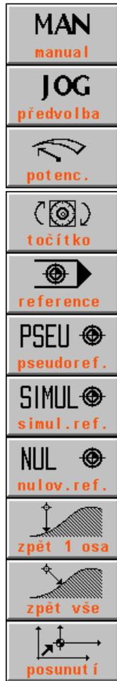
Manual travel mode for all axes generally. After pressing down the push-button the F1 up to F6 push-buttons became functions push-buttons for negative movement directions.
