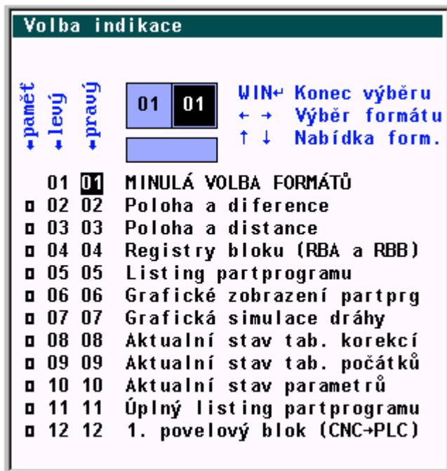
In the right window, the list of possible formats is displayed (see the Figure). The left window remains unchanged. When a format exists only in one window before pressing down the WIN push-button, it will be reduced to its half size and displaced into the left window.
