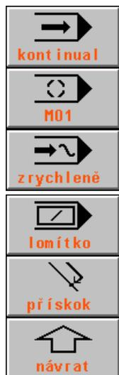
AUT mode with the BB modification (“block by block”). After selection of it, the part program run will be stopped after block finishing.
